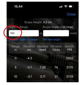
On the top right, you will see the **calculated scope angle** for your current elevation turret position, which in this example is 1.24mrad. You can round this value to 1.2mrad if you want, since it is not possible to adjust the elevation turret in increments of 1/10th of a click. Once you have the calculated scope angle, set it to the scope angle field and use it instead of the sight-in range.
