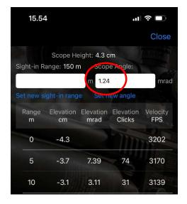
The advantage of using the scope angle instead of the sight-in range is that you can shoot any bullet and get a correct ballistic solution regardless of the actual sight-in range for the bullet. **The elevation clicks reported in the app are based on the elevation turret zero position**. This means that by using the scope angle instead of the sight-in range, you can shoot any bullet and get a correct solution without needing to adjust the sight-in range for each bullet. **FX**outdoors
