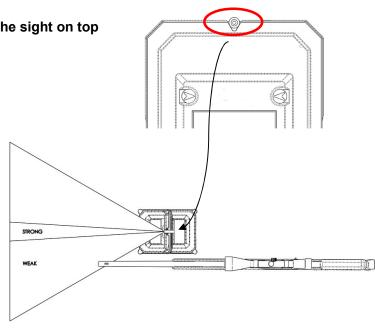
cone is important because it determines the area that the radar can detect and the direction in which it can detect objects. Because the strong signal emitted by the chronograph is very narrow, it is important to **aim the device carefully** for accurate results. The weak signal is also important, as it is used for **triggering the chronograph**. When the bullet enters the radar cone (indicated by the weak signal), the chronograph is triggered.
