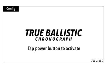
After pressing the Config button, you will be taken to a page with the Velocity Range at the top. Since the current firmware only has one velocity range to choose from (400 FPS - 4000 FPS), this option will not be shown.
